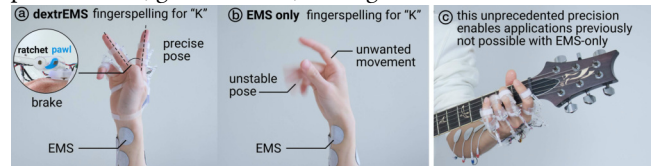
Figure 3: DextrEMS increases dexterity of EMS by combining it with brakes.
